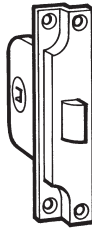
BRASS BOLT AND FOREND HALF REBATED FOREND 157 x 27 x 13mm. STEEL CASE DEPTH 75mm. HEIGHT 70mm. THICKNESS 14mm BACKSET 60mm 95-658 REBATED MORTICE LATCH
