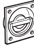
ALUMINIUM, CAST, 65 x 65mm. WHEN USED WITH 95-658 MORTICE LATCH MINIMUM DOOR THICKNESS 38mm S.A.A. 95-631 FLUSH RING HANDLE
