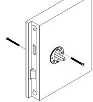
Fix the rose mounting plates (metal) to door and secure with the M4 bolt through fixings
