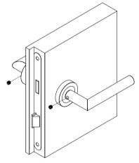
Tighten the grub screws on both levers ensuring they pierce the spindle.
