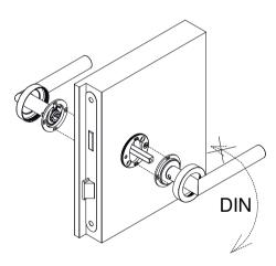
Place the lever base rose on the spindle and push onto the mounting plates. Pay attention to the direction of the lever handles ensuring they can be pressed downwards.
