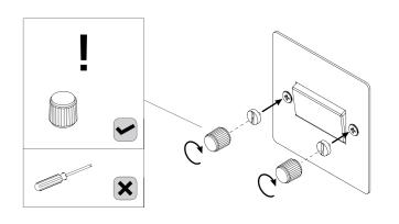
\*\* Do NOT use a standard screw driver to tighten the coin caps. This may damage the cap and is not covered under warranty. Plastic coin cap tool must be used by hand only.
