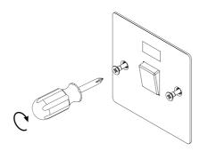
\* Please ensure screws are sufficiently tight to support the product but please do not over tighten as this may cause some deformation to the plate or damage the
