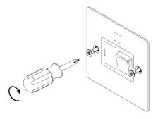
\* Please ensure screws are sufficiently tight to support the product but please do not over tighten as this may cause some deformation to the plate or damage the screw.
