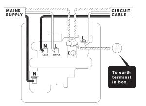
\* This fused connection unit is fitted with two linked terminals to provide a dual earth facility. This is for use in "clean earth" installations were additional earth capacity is required to comply with regulation 607 of BS 7671 IET wiring regulations.
