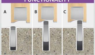
SOFT / MEDIUM CONTROLLED OPENING STRENGTH, HOLD OPEN IS ACTIVATED.
