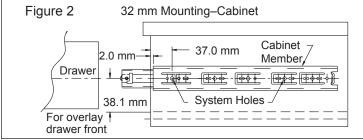
2. Use only the 32 mm system holes or the wood screw holes located at the tip of the breathing tabs. Do not use any other holes on the cabinet member for mounting (Figure 3).
