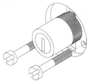
From the inside of the door insert the two metal thread screws through the lock case & screw into the outside rose. Do not over tighten.
