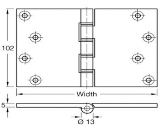
Projection hinges are drilled with holes towards the edge of a broad hinge leaf enabling the hinge to clear obstructions when fully open beyond 90 degrees
