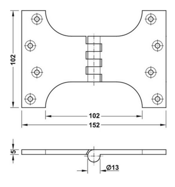
Projection hinges are drilled with holes towards the edge of a broad hinge leaf enabling the hinge to clear obstructions when fully open beyond 90 degrees
