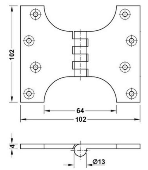
Projection hinges are drilled with holes towards the edge of a broad hinge leaf enabling the hinge to clear obstructions when fully open beyond 90 degrees
