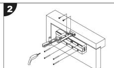
Using the templates provided, fix the mechanism to the door as well as the armset and any necessary brackets
