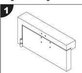
Using the templates provided, mark and drill pilot holes into the door and frame
