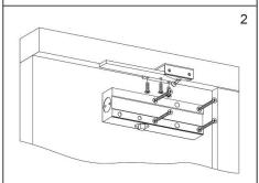
Using the templates provided, fix the mechanism to the door as well as the armset and parallel arm bracket.
