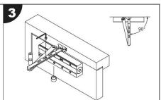
Attach the armset to the mechanism ensuring the pre-loading requirement has been completed
