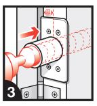
Drill the hole for the closer body using the Lewis auger bit.
