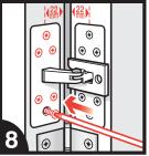
Fix the plate onto the door frame making sure it is exactly in line with the other plate.
