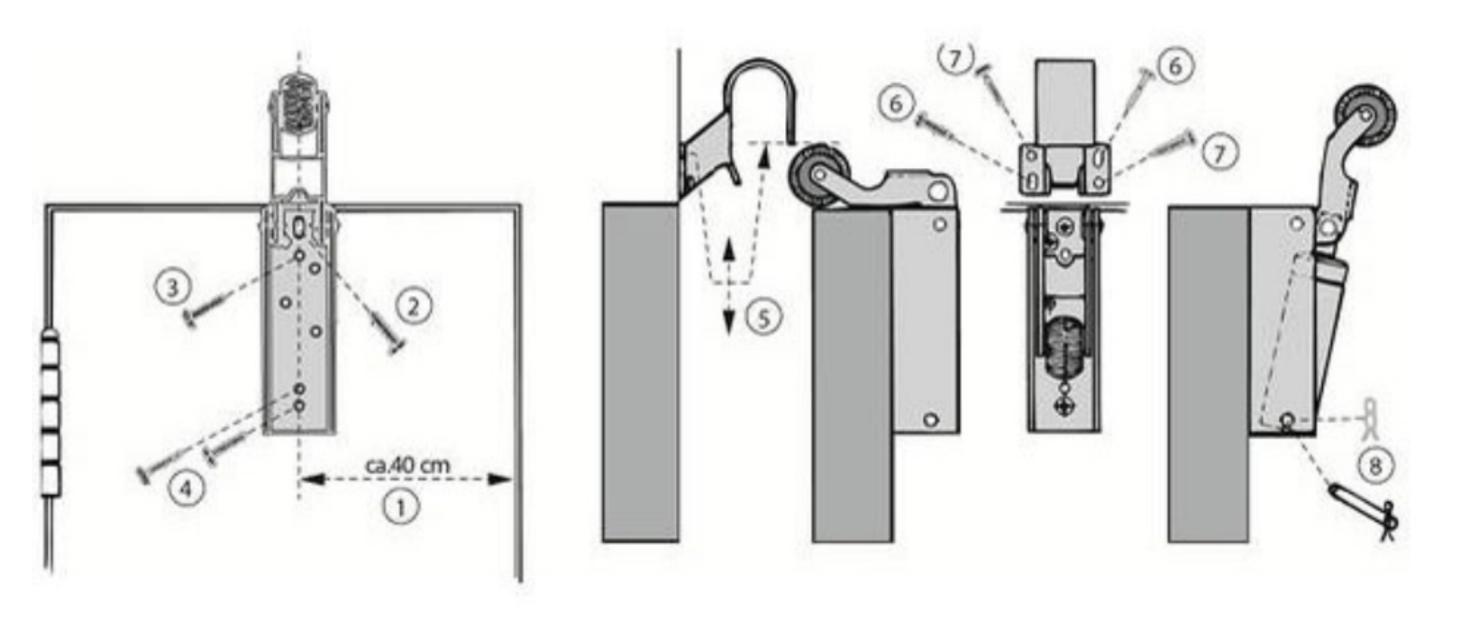
The DICTATOR door damper Z 1000 is fixed vertically more or less in the centre of the door leaf. The upper edge of the casing should stand out about 1 mm from the upper edge of the door leaf. See drawing under 'Dimensions'.
