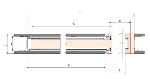
A Passage width I B Passage height I C Door width I D Door height I E Overall width I F Overall height I G Frame width I H Passage size without jambs I I Height from finished floor to inside face of track I J Finished wall I Y Interior width I K Max. door thickness I W Frame thickness
