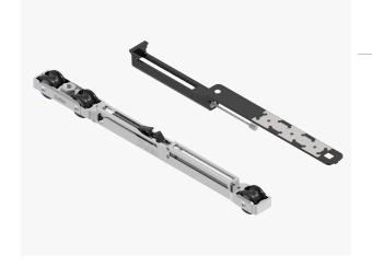
Provides a soft closing and opening of the door. It retains the door in the last 10cm of its sliding path, holding it in a controlled way until the end of its journey and avoiding slams as well as extending the useful life of the product.
