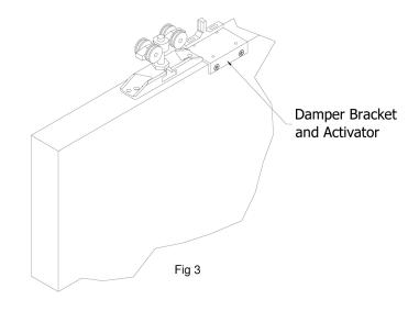
WARNING! DO NOT APPLY ANY ADDITIONAL SUBSTANCES, LUBRICANTS ETC. TO THE DAMPER. DOING SO MAY DAMAGE THE PRODUCT AND VOID THE WARRANTY.
