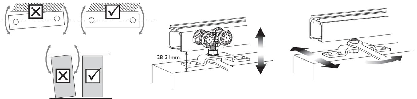
**6 Once positioned, secure the soft stop block to the track by tightening the grubscrews. Secure the bracket to the underside of the track by tightening the bolts**
