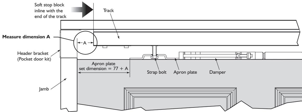
**I With the offset in mind - secure the damper and hanger to the top of the door**
