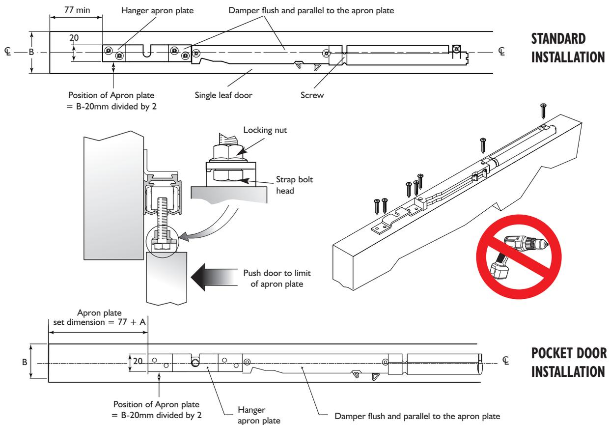
**2 Sub assemble the bracket and block with the fixings supplied**
