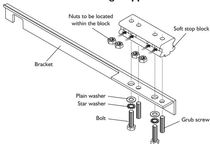
**3 Locate the sub assembled bracket into the end of the track**
