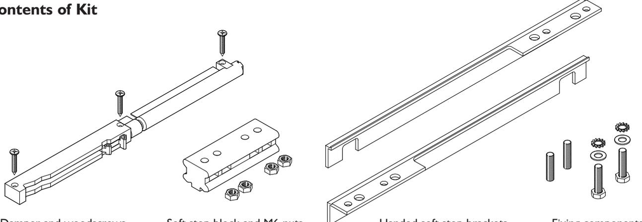
Damper and woodscrews      Soft stop block and M6 nuts      Handed soft stop brackets      Fixing components
