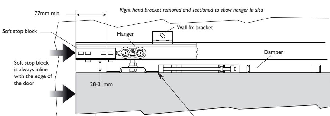
77mm min      Right hand bracket removed and sectioned to show hanger in situ      Wall fix bracket      Damper
