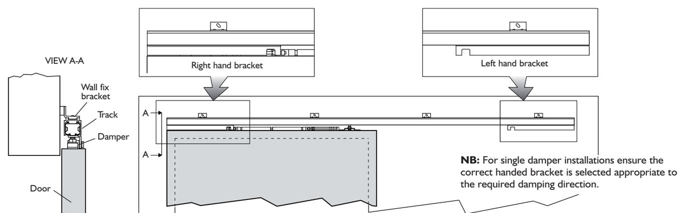
**NB:** For single damper installations ensure the correct handed bracket is selected appropriate to the required damping direction.
