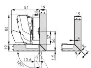
With 0 cranking, mounting plate height 19 mm and cup distance 4 mm, door and cabinet edges can meet at mitred angles on all 4 sides.
