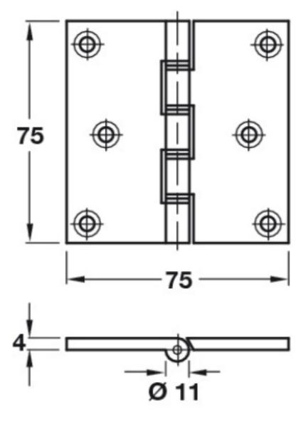
Projection hinges are drilled with holes towards the edge of a broad hinge leaf enabling the hinge to clear obstructions when fully open beyond 90 degrees
